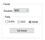
Select the baud rate and required parity and press the Set address button.
