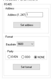
The address of each Paladin Advantage can be set to any value between 1 and 247.
