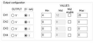
The output values can be V or mA. Should a mid point be selected in the parame-
